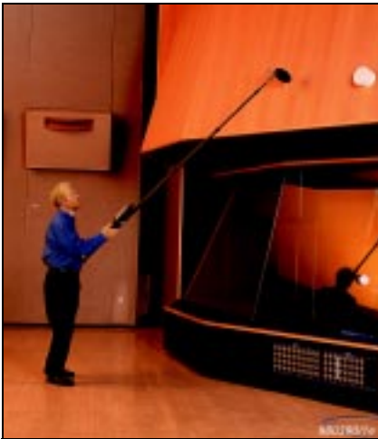
Fig. 22 Mapping the sound reduction to find leakages between studio and control room
